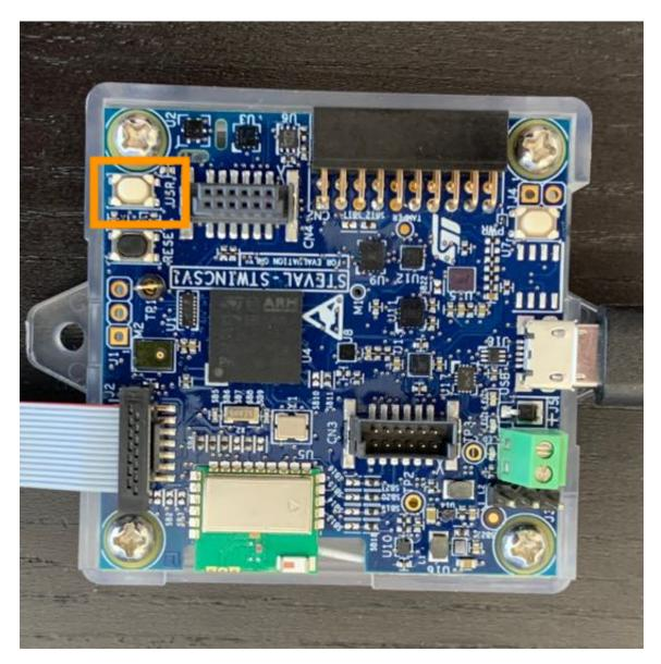
1. While holding the USR button, connect STWINK1B to the other end of the micro-USB cable.
